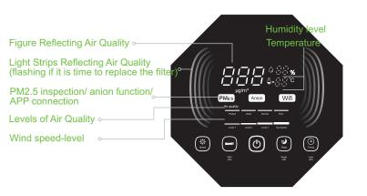
Start Button: When the air purifier is powered up, the "Start button" turns red, and enters the standby mode; press the button to start the machine; the standby-mode power consumption is less than 2W; separate the machine from its source of power to shut it down completely (Note: in the smart mode, anion function runs automatically, and sensor begins to inspect the machine).
